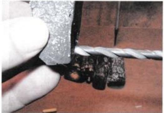
15. Cut a Q-Tip in half and use the stick end to apply Pyrofix glue to the drilled holes. Push the pins into the glue and clean up any excess glue with the fuzzy end of the Q-Tip.
