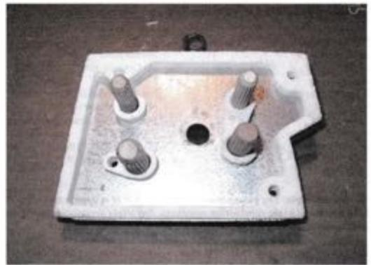
Carefully place the ember bed over the dowels making sure the teardrop shaped gasket doesn't slip out of place.
